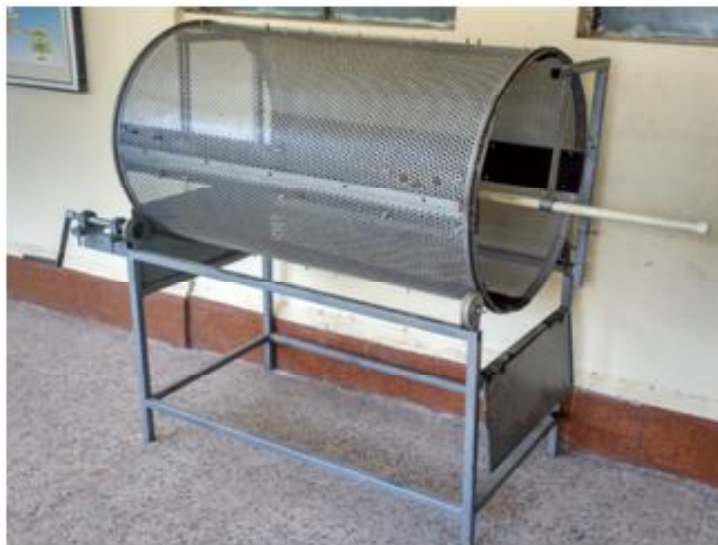
Plate 1: Final design of the hand operated root crop washer
