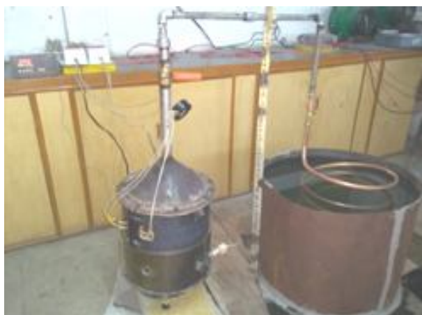
Fig2. Pyrolytic reactor system for fuel oil recovery from wasteplastics
